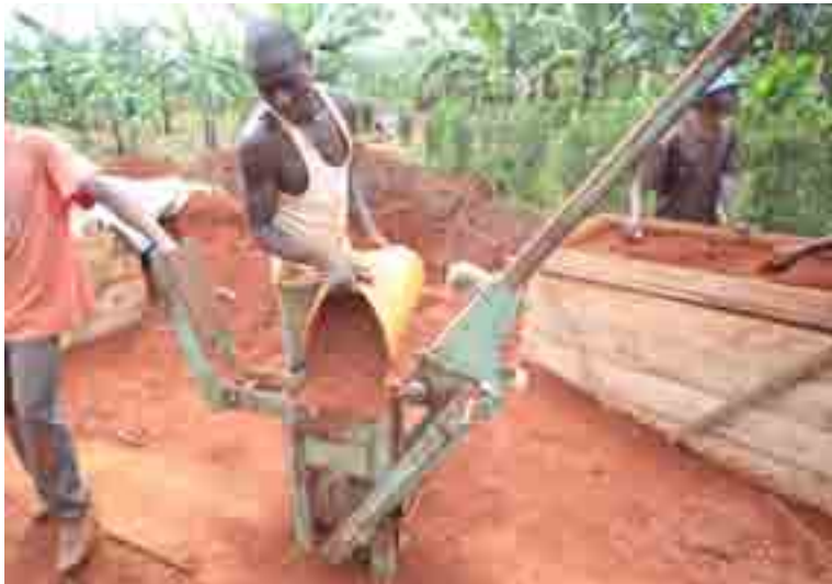
(2) Sifted soil is poured into the earth block press. A stabilizer can be added to the mixture to produce a SCEB.
