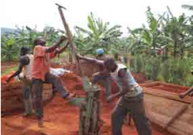
(3) Compressing the mixture manually by two people.
