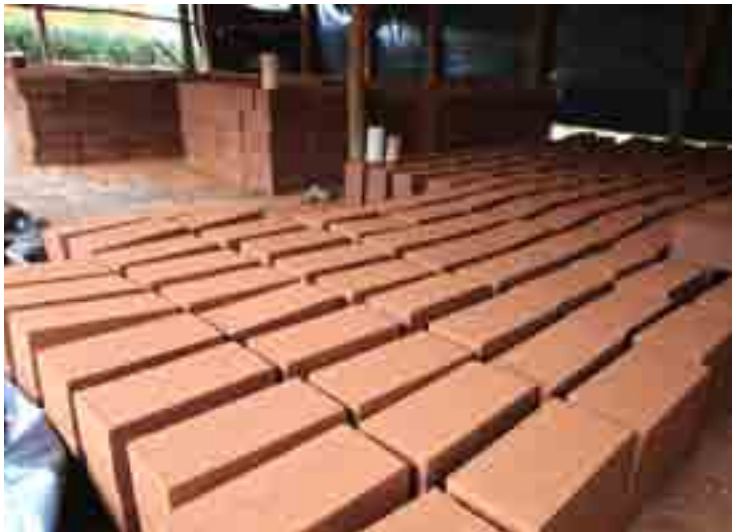
(5) Curing / Drying the blocks is done for a period of four weeks after manufacturing.
